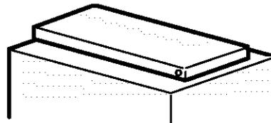
2.6 Transfer the 2 screws from the opposite side of the cabinet to the screw holes vacated by the top hinge removal.
