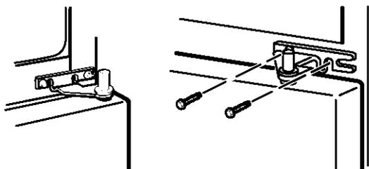
3.3 Remove the tape and tilt the door away from the cabinet. Lift the door from the pin in the bottom hinge bracket. (If the plastic washer sticks to the door bottom, put it back on the hinge.)
