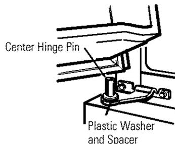
6.2.2 Tilt the door toward the cabinet, lifting the top hinge so the pin fits into the socket on the top of the door.
