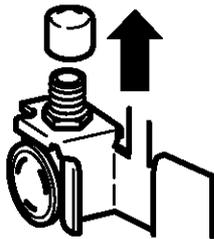
Place the compression nut and ferrule (sleeve) onto the end of the tubing as shown. On GE SmartConnect™ Refrigerator Tubing kit, the nuts are already assembled to the tubing.
