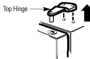
2.4 Remove the tape and tilt the door away from the cabinet. Lift it off the center hinge pin.
