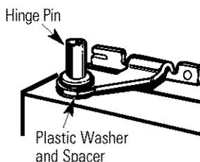
6.1.3 Tilt the door toward the cabinet. As the door is brought into position, slide the hinge under the head of the screw which earlier had been partly driven into the outermost hole. Insert the remaining screw, then tighten both screws securely.
