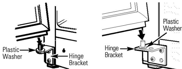
Models with a hinge bracket that has 2 screw holes.
