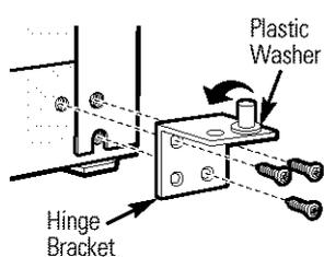
Models with a hinge bracket that has 4 screw holes.
