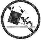
To reduce the risk of tipping, the range must be secured by properly installed anti-tip bracket(s) provided with the range. To check if the bracket(s) is installed properly, remove the lower panel or storage drawer and verify that the anti-tip bracket(s) is engaged. Refer to the Installation Instructions for proper anti-tip bracket(s) installation.
