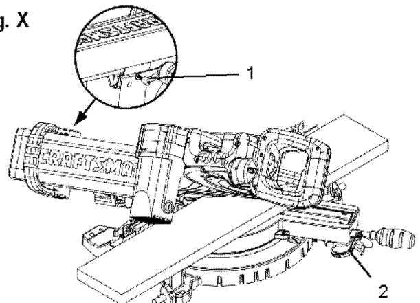
**NOTE:** The saw comes with a 33.9° bevel detent pin for setting up crown molding cuts.
