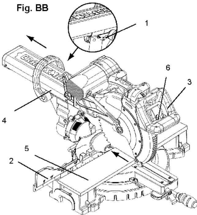
2. Lower the cutting head so the tip of the blade touches the top surface workpiece at the marked line.
