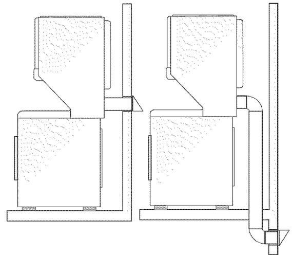
4. When installing a gas dryer into a mobile home, a provision must be made for outside make up air. This provision is to be not less than twice the area of the dryer exhaust outlet.
