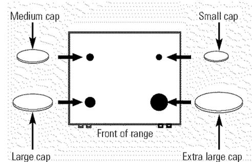
Make sure that the heads and caps are replaced in the correct locations.
