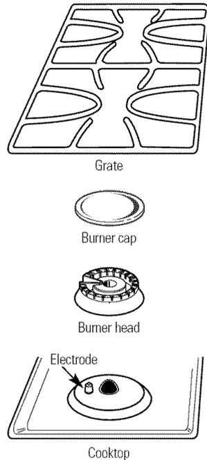
Place burner heads over the electrodes on the cooktop, in the correct locations according to their size.
