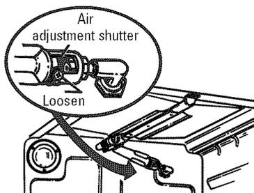
The air adjustment shutter for the top (broil) burner is in the center of the rear wall of the oven.
