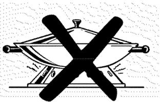
Do not use a flat-bottomed wok on a support ring. Placing the ring over the burner or grate may cause the burner to work improperly, resulting in carbon monoxide levels above allowable standards. This could be dangerous to your health.
