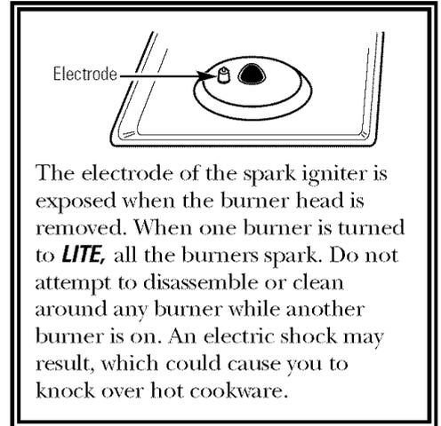
The electrode of the spark igniter is exposed when the burner head is removed. When one burner is turned to **LITE**, all the burners spark. Do not attempt to disassemble or clean around any burner while another burner is on. An electric shock may result, which could cause you to knock over hot cookware.
