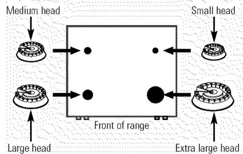
Make sure the slot in the burner head is positioned over the electrode.
