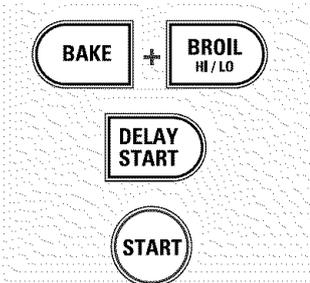
With this feature, should you forget and leave the oven on, the control will automatically turn off the oven after 12 hours during baking functions or after 3 hours during a broil function.
