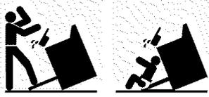
If your range is removed for cleaning, servicing or any reason, be sure the anti-tip device is re-engaged properly when the range is replaced. Failure to take this precaution could result in tipping of the range and cause injury.
