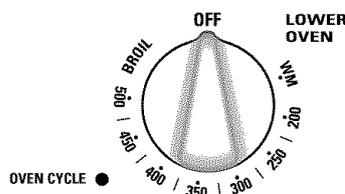
The **OVEN CYCLE** light glows until the oven reaches your selected temperature, then goes off and on with the oven element(s) during cooking.
