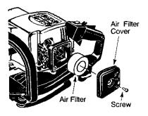
A dirty air filter decreases engine performance and increases fuel consumption and harmful emissions. Always clean after every 5 hours of operation.
