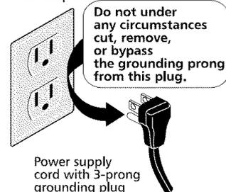
Power supply cord with 3-prong grounding plug
