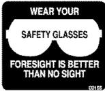
The operation of any tractor can result in foreign objects thrown into the eyes, which can result in severe eye damage. Always wear safety glasses or eye shields while operating your tractor or performing any adjustments or repairs. We recommend a wide vision safety mask over spectacles or standard safety glasses.
