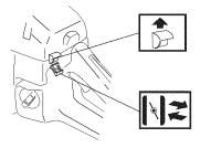
Use the same procedure as for starting a cold engine but without setting the choke control in the choke position. The correct choke/start throttle setting is obtained by moving the choke control to the choke position and then pushing it in again.
