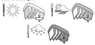
An air filter that has been in use for a long time cannot be cleaned completely. The filter must therefore be replaced with a new one at regular intervals. A damaged air filter must always be replaced.
