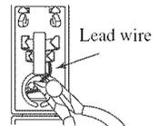
**4** Insert the cable wire into the slot, and clamp it with pliers.
