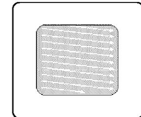
The progressive scanning method scans one full frame of video consecutively down the screen, line by line. An entire image is drawn at one time, as opposed to the interlaced scanning process by which a video image is drawn in a series of passes. The progressive scanning method is desirable for dealing with moving objects.
