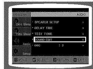
**4** Press Cursor **▲**, **▼** buttons to select and adjust the desired item. Press the **◀**, **▶** buttons to adjust the settings.
