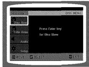
**2** Press Cursor **▼** button to move to 'Setup' and then press **ENTER** button.
