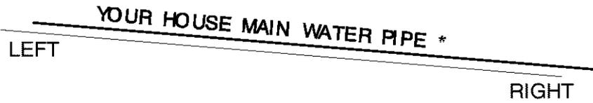
\* In what direction does the water flow? Be sure to plan IN and OUT piping so water flow is to the softener valve inlet. Plan a crossover if flow is from left to right.
