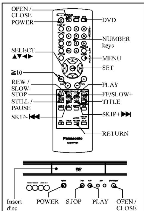
If a remote control button does not work when pressed, press the DVD button on the remote and try the button again.
