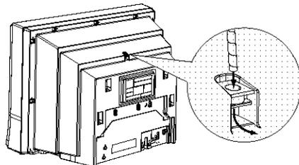
The unit may tip or fall if not situated on a stable surface, if pushed, or during an earthquake. Use a strong rope or chain (not included) to fasten the unit firmly to a strong wall support.
