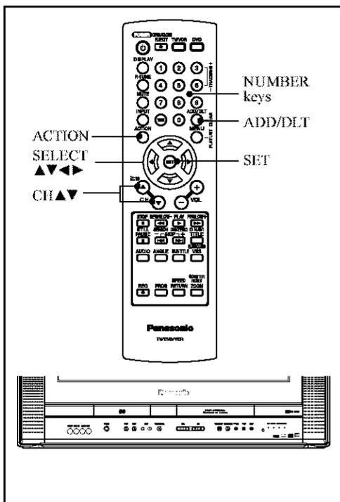
4 Press ▲▼ to select “ANTENNA,” then press SET to set your antenna system (“TV” or “CABLE”).
