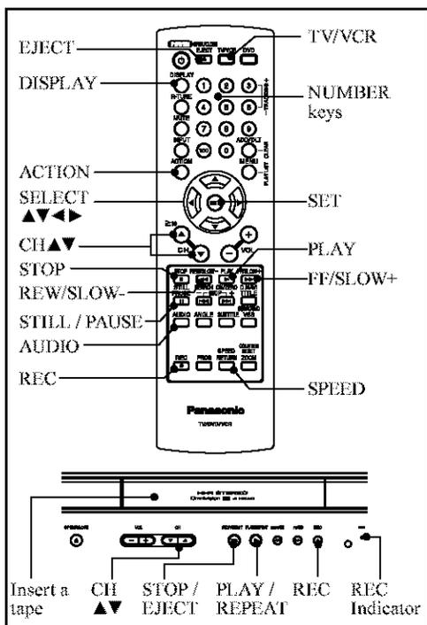
If a remote control button does not work when pressed, press the TV/VCR button on the remote and try the button again.
