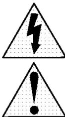
This symbol warns the user that uninsulated voltage within the unit may have sufficient magnitude to cause electric shock.
