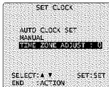
3 Press **▲▼** to select "TIME ZONE ADJUST" and press **SET** to subtract or add hour(s) as necessary.
