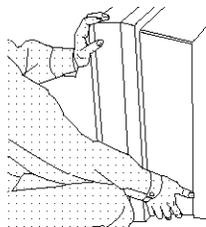
Always grasp bottom and front of unit as shown for proper balance.
