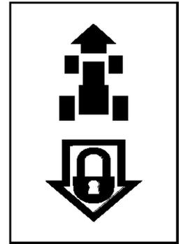
**NOTE:** Cruise control can not be engaged at the tractor's fastest ground speed. If the operator should attempt to do so, the tractor will automatically decelerate to the fastest optimal mowing ground speed.
