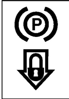
**NOTE:** The parking brake must be set if the operator leaves the seat with the engine running or the engine will automatically shut off.
