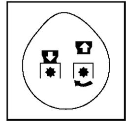
**NOTE:** The PTO knob **must** be in the disengaged (OFF) position when starting the engine, when traveling in reverse and if the operator leaves the seat.
