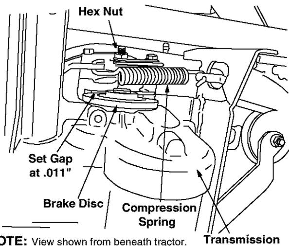
**NOTE:** View shown from beneath tractor. Transmission
