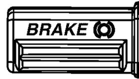
The brake pedal is located on the right front side of the tractor above the drive pedal along the running board. The brake pedal can be used for sudden stops or for setting the parking brake.
