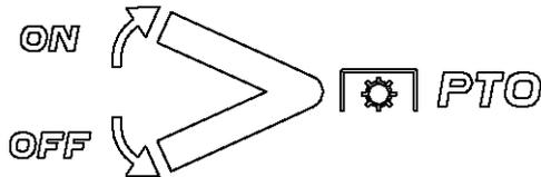
The PTO lever is located on the left side of the dash next to the steering wheel. Move the PTO lever forward to engage the power to the cutting deck or other attachments; move the PTO lever backward (toward the rear of the tractor) to disengage the power to the attachments.
