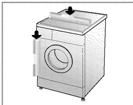
1. Leveling a the washing machine properly prevents excessive noise and vibration. Install the appliance on a solid and level floor surface, preferably in a corner of the room.
