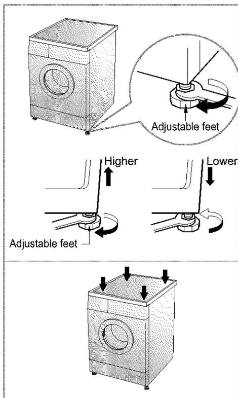
2. If the floor is uneven, adjust the adjustable feet as required. (Do not insert pieces of wood, etc. under the feet)
