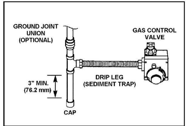
FIGURE 19. GAS PIPING WITH FLEXIBLE CONNECTOR.
