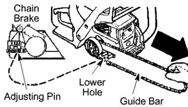
13. Install chain brake nuts and finger tighten only. Do not tighten any further at this point. Proceed to CHAIN ADJUSTMENT.
