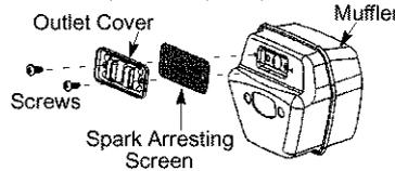
6. Clean the spark arresting screen with a wire brush. Replace screen if any wires are broken or screen is blocked after cleaning.
