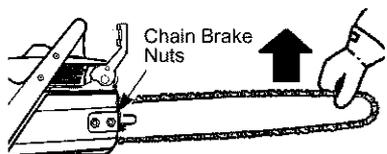
7. Use the screwdriver end of the bar tool to move chain around guide bar.
