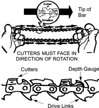
8. Place chain over and behind clutch, fitting the drive links in the clutch drum sprocket.
