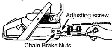
4. Using bar tool, roll chain around guide bar to ensure all links are in bar groove.
