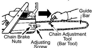
2. Loosen chain brake nuts until they are finger tight against the chain brake.
