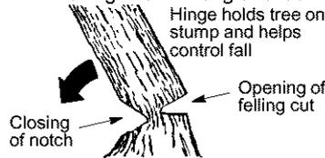
**NOTE:** Before felling cut is complete, use wedges to open the cut when necessary to control the direction of fall. To avoid kickback and chain damage, use wood or plastic wedges, but never steel or iron wedges.
