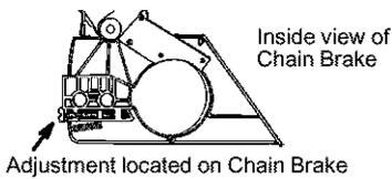
5. Turn adjusting screw by hand counterclockwise until adjusting pin just touches the stop.
