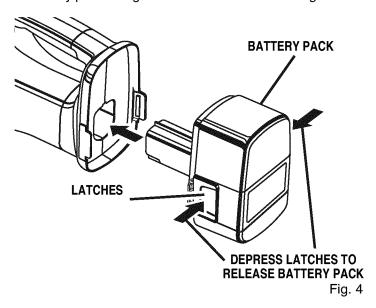
Make sure the latches on each side of battery pack snap into place and battery pack is secured in hand vac before beginning operation.
