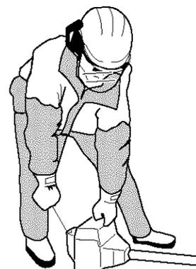
NOTE! Do not pull the starter cord out completely and do not release the starter cord from the fully extended position. This can damage the hedge trimmer.
