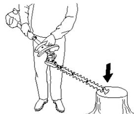
**NOTE! Do not hold the cutting attachment when you adjust the angle. The blades are sharp and you could easily cut yourself.**
