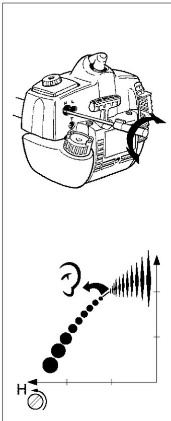
Therefore dismantle the cutting equipment, nut, support flange and disc drive before adjusting the high speed needle. The high speed needle is adjusted correctly when the machine 'splatters' a little .
