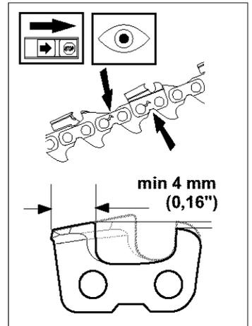
When the length of the cutting teeth has worn down to only 4 mm the chain must be replaced.
