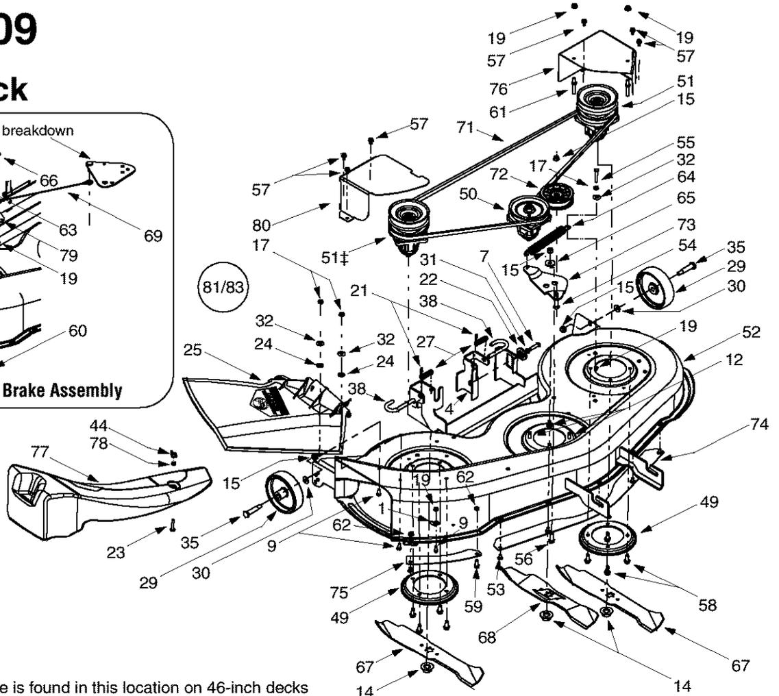
‡ A double-pulley spindle is found in this location on 46-inch decks engaged by electric PTOs only. Use 618-0240 on manual PTO decks.
