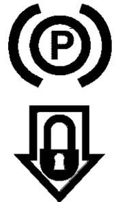
**NOTE:** The parking brake must be set if the operator leaves the seat with the engine running or the engine will automatically shut off.
