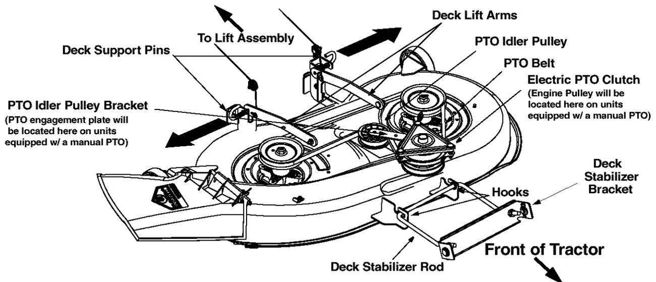
**NOTE:** Belt covers and other tractor components not shown for clarity. 42-inch deck shown
