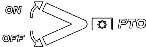
The PTO lever is located on the left side of the dashboard next to the steering wheel. Move the PTO lever forward to engage the power to the cutting deck or other attachments; move the PTO lever backward (toward the rear of the tractor) to disengage the power to the attachments.
