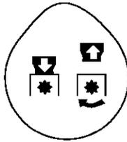
**NOTE:** The PTO knob **must** be in the disengaged (OFF) position when starting the engine, when shifting into reverse and if the operator leaves the seat.
