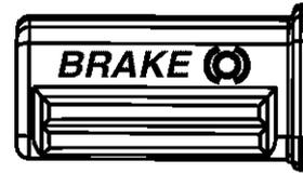
The brake pedal is located on the right front side of the tractor above the drive pedal along the running board. The brake pedal can be used for sudden stops or setting the parking brake.
