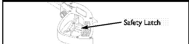
Figure 8 — Spray Gun with Safety Latch Engaged
