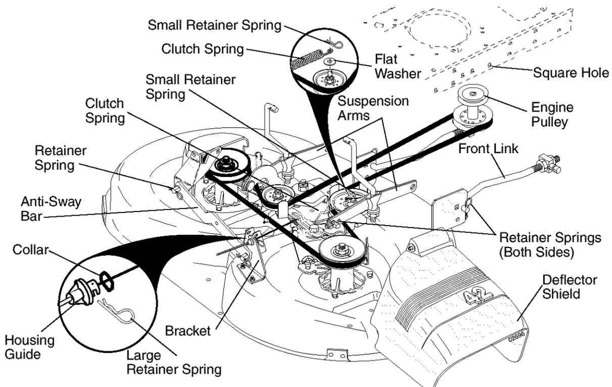
7. Push clutch cable housing guide into bracket, slide collar onto guide and secure with large retainer spring.
