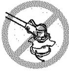
**⚠ WARNING:** The blade continues to spin after throttle is released or engine is turned off. The coasting blade can throw objects or seriously cut you if accidentally touched. Stop the blade by contacting the left hand side of coasting blade with material already cut.
