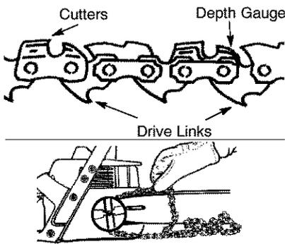
Place chain onto the sprocket
