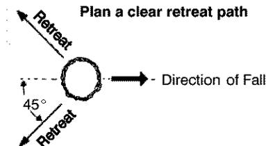
**WARNING:** Do not cut near buildings or electrical wires if you do not know the direction of tree fall, at night since you will not be able to see well, or during bad weather such as rain, snow, or strong winds, etc.
