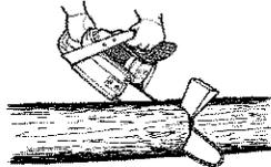
Turn saw OFF and use a plastic or wooden wedge to force cut open.
