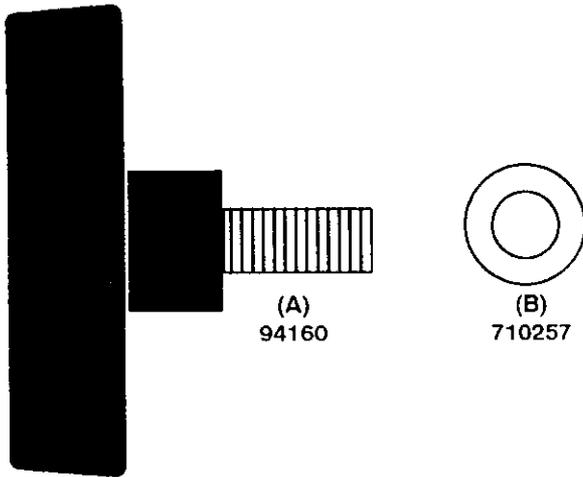
3. Check the operating position of the **seat**. If the **seat** needs to be adjusted, loosen the two **wing bolts**. Slide the **seat** forward or backward along the **seat adjusting holes** as shown. Tighten the **wing bolts (A)**.
