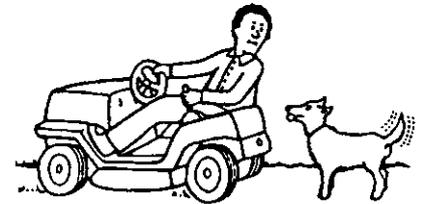
Before you leave the mower, stop the engine. Remove the key. Disengage and lower any attachment. Set the parking brake. Never mount or dismount from the seat while the engine is running. An accident can occur if you touch the brake, speed control pedal, throttle, or blade control while the engine is running. Mount and dismount from the seat on the side of the unit that is marked ENTER-EXIT.
