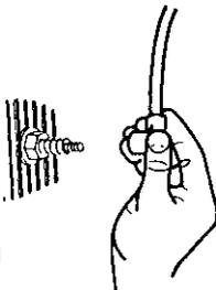
If you hit a large object during operation, stop the engine. Remove the wire from the spark plug. Carefully inspect the mower for damage. Before you start the engine again, make the necessary repairs. If you
