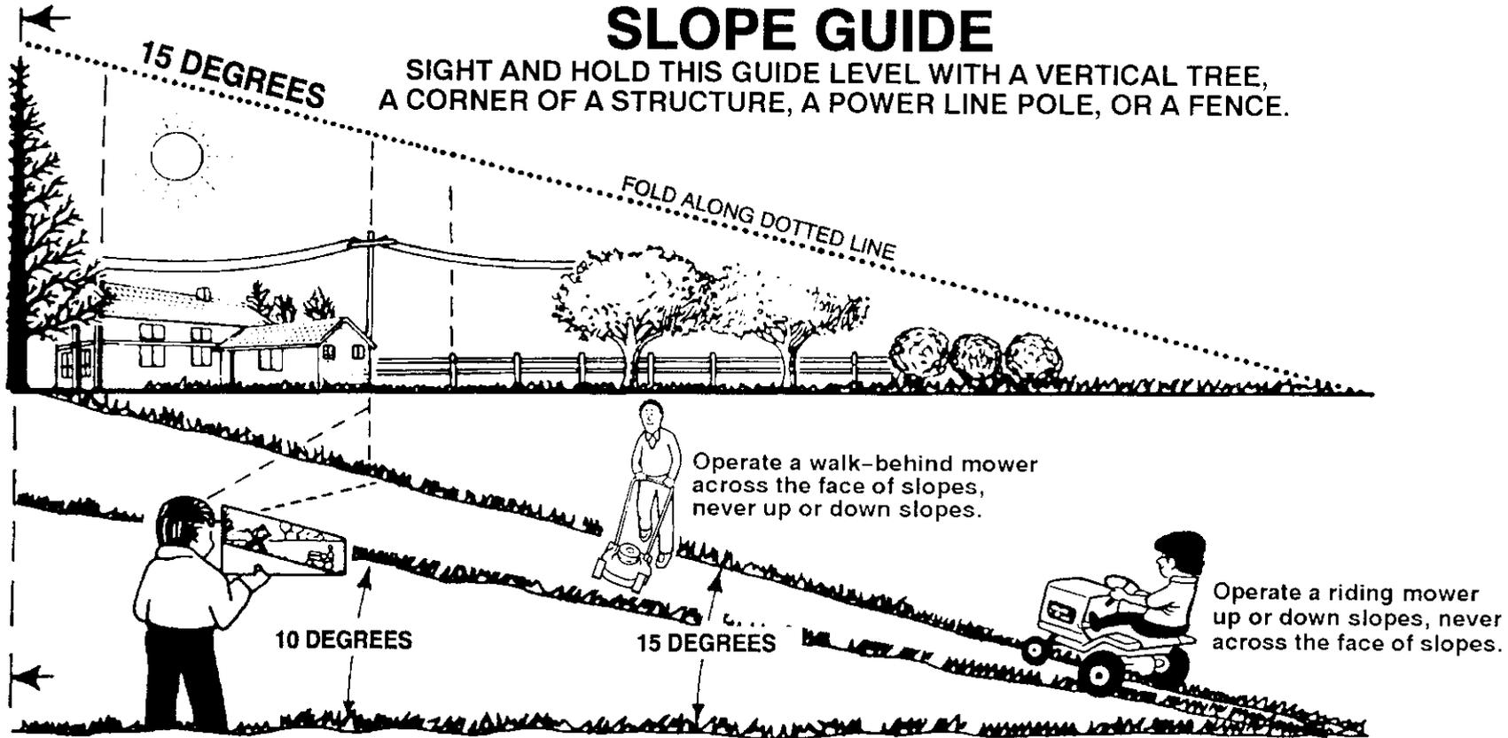
On a riding mower to determine if a slope is safe to mow: (1) disengage the blade(s), (2) put the unit in reverse, and (3) try to back straight up the slope. If you can back up the slope, it is generally safe to mow. However, if you do not feel safe, or if you are not completely sure, use this guide and do not mow a slope that is greater than 15 degrees. If the riding mower is used with a pull-behind or rear mounted attachment, do not operate the unit on a slope that is greater than 10 degrees.
