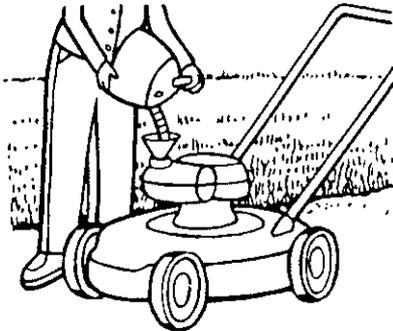
If you add gasoline to an engine that is running or hot, the result can be an explosion. Before you add gasoline, stop the engine and let the engine cool for several seconds. Remove dry grass and other debris from the mower. Keep the mower clean to improve the performance, help the engine and transmission run cooler, extend the life of moving parts, and decrease the danger of a fire.
