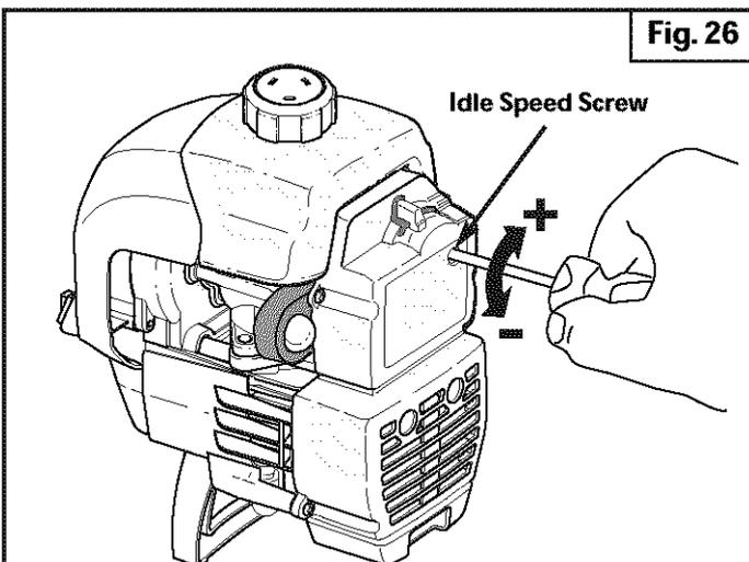
3. If the engine appears to be idling too fast, turn the idle speed screw **counterclockwise** 1/8 of a turn at a time (as needed), to reduce idle speed.
