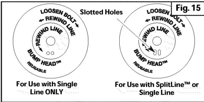
**NOTE:** SplitLine™ can only be used with the inner reel with the slotted holes. Single line can be used on either type of inner reel. Use Figure 15 to identify the inner reel you have.
