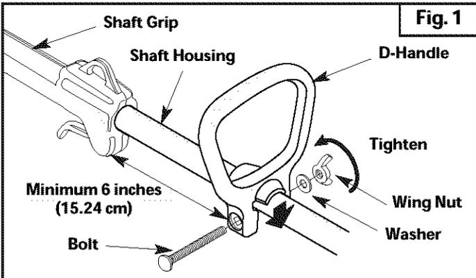
2. Insert the shoulder bolt into the squared hole in the handle and push through. On the left side of the handle, place the washer on the bolt, then screw the wing nut onto the bolt. Do not tighten until you make the handle adjustment.
