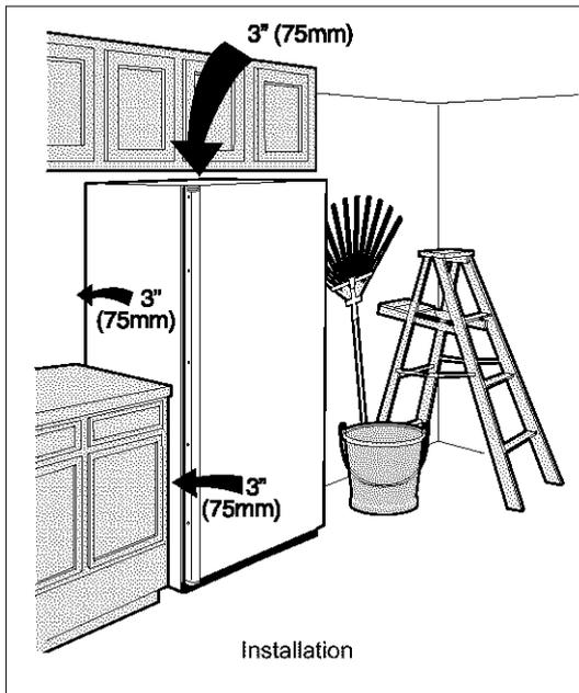
**NOTE:** The exterior walls of the refrigerator may become quite warm as the compressor works to transfer heat from the inside. Temperatures as much as 30° F warmer than room temperature can be expected. For this reason it is particularly important in hotter climates to allow enough space for air circulation around your refrigerator.
