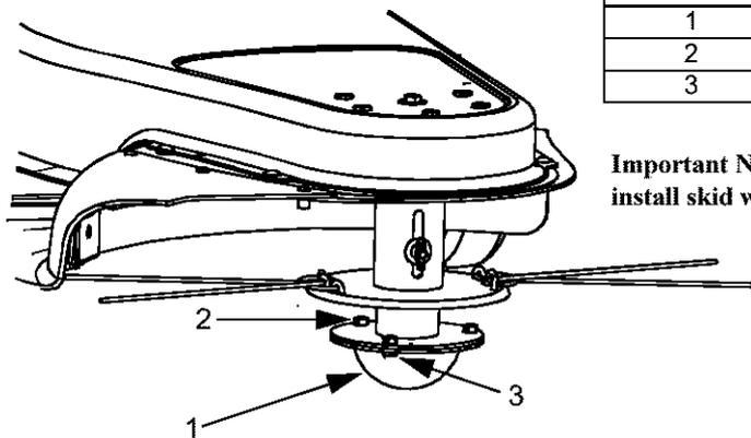
**Important Note: When replacing Trimmer Skid discard the original hardware and install skid with new hardware provided. Hardware is not to be reused.**
