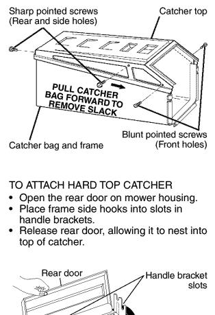
**ACAUTION:** Under normal usage, the catcher material is subject to deterioration and wear and should, therefore, be checked frequently for replacement. Any replacement catcher should be checked to ensure compliance with original manufacturer's specifications.
