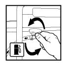
Move the choke control located on the engine to "CHOKE" position. A cold engine may require to be choked longer than a warm engine.
