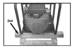
7. On the muffler side of the engine, remove cap screws and flange nuts holding the heat shield to the frame. Reassemble cap screws, heat shield, wheel bracket, and flange nuts and as shown. Tighten securely.
