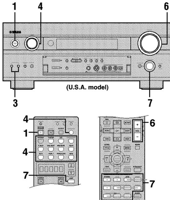
**1 Press STANDBY/ON (SYSTEM POWER on the remote control) to turn on the power.**
