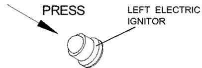
8. If the burner does not light, turn the Control Knob to OFF, wait 5 minutes for gas to clear, then retry.
