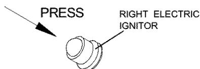
8. If the burner does not light, turn the control knob to OFF, wait 5 minutes for gas to clear, then retry.
