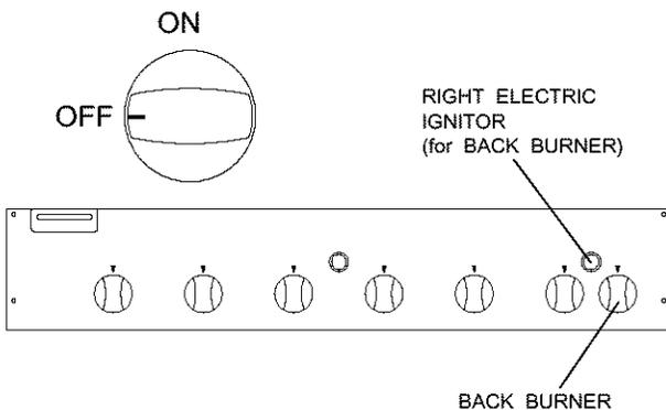
7. Immediately press the Right Electric Ignitor for 3-4 seconds to light the Back Burner.
