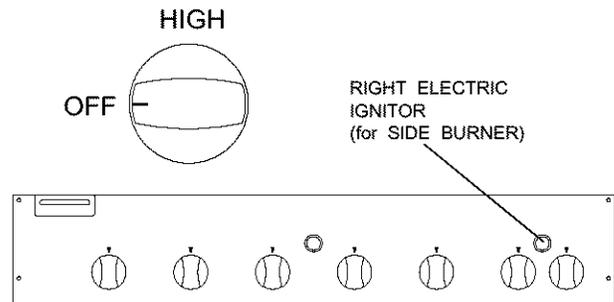
3. Immediately press the right electric ignitor for 3-4 seconds to light the burner.
