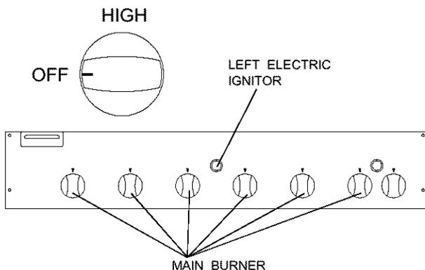
7. Immediately press the left Electric Ignitor for 3-4 seconds to light the Burner.
