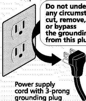
Do not under any circumstances cut, remove, or bypass the grounding prong from this plug.
