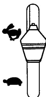
**GB** Warm motor: Push the gas control half-way to full gass position "▲".
