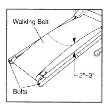
wrench, turn both rear roller adjustment bolts counterclockwise 1/4 of a turn. When the tension of the walking belt is correct, you should be able to lift each side of the walking belt 2 to 3 inches. Walk on the treadmill for a few minutes. Repeat until the walking belt is properly tightened. Be careful to keep the walking belt centered.
