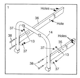
Raise the Left Upright (35) and the Right Upright (36) to the position shown. Feed the Reed Switch Wire (6) into the top of the Left Upright and out of the indicated hole.
