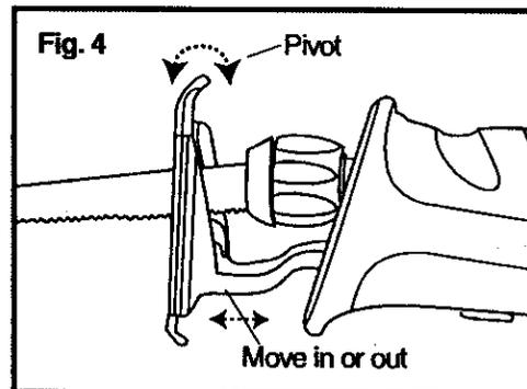
**NOTE:** The shoe also pivots to provide maximum control against the surface being cut.
