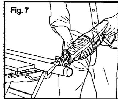
**NOTE:** We recommend that you spread a thin film of oil or other coolant along the line of cut ahead of the saw. This will allow easier operation and help extend blade life. When cutting aluminum, use kerosene.
