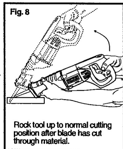
**NOTE:** In areas where blade visibility is limited, use the edge of the saw guard as a guide.
