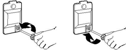
3. Turn bulb counterclockwise. Replace the bulb only with a 10-watt appliance bulb. Replace the cover and secure with the screw.
