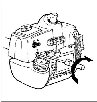
**CAUTION!** Contact your servicing dealer, if the idle speed setting cannot be adjusted so that the cutting attachment stops. Do not use the machine until it has been properly adjusted or repaired.
