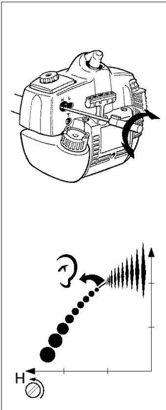
Therefore dismantle the cutting equipment, nut, support flange and disc drive before adjusting the high speed needle. The high speed needle is adjusted correctly when the machine 'splatters' a little. If the machine smokes heavily at the same time as it 'splatters' heavily the adjustment is too rich.
