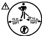
The operator of the machine shall ensure, while working, that no persons or animals come closer than 15 metres.
