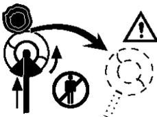
Blade can thrust violently when coming in contact with any object. Blade thrust can cause amputation of arms or legs. Keep people and animals 50 feet away. Never use blades unless recommended handlebar, shoulder strap, attaching hardware and blade deflector are installed.
