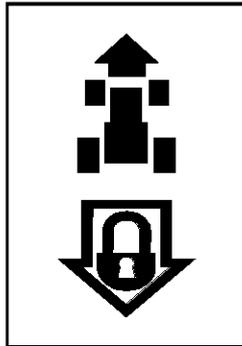
**NOTE:** Cruise control can NOT be engaged at the tractor's fastest ground speed. If the operator should attempt to do so, the tractor will automatically decelerate to the fastest optimal mowing ground speed.
