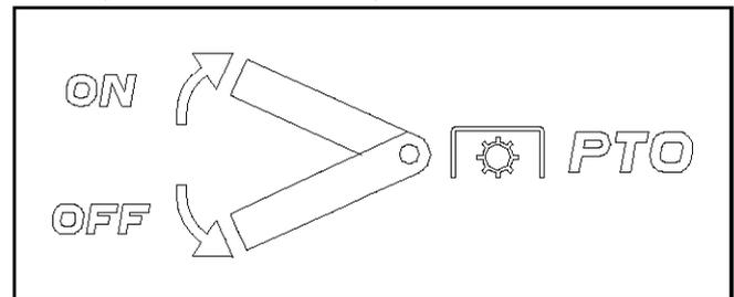
On models equipped with a manual PTO, the PTO lever is located on the left side of the dashboard next to the steering wheel. Move the PTO lever forward to engage the power to the cutting deck or other (separately available) attachments; move the PTO lever rearward to disengage the power to the attachments.
