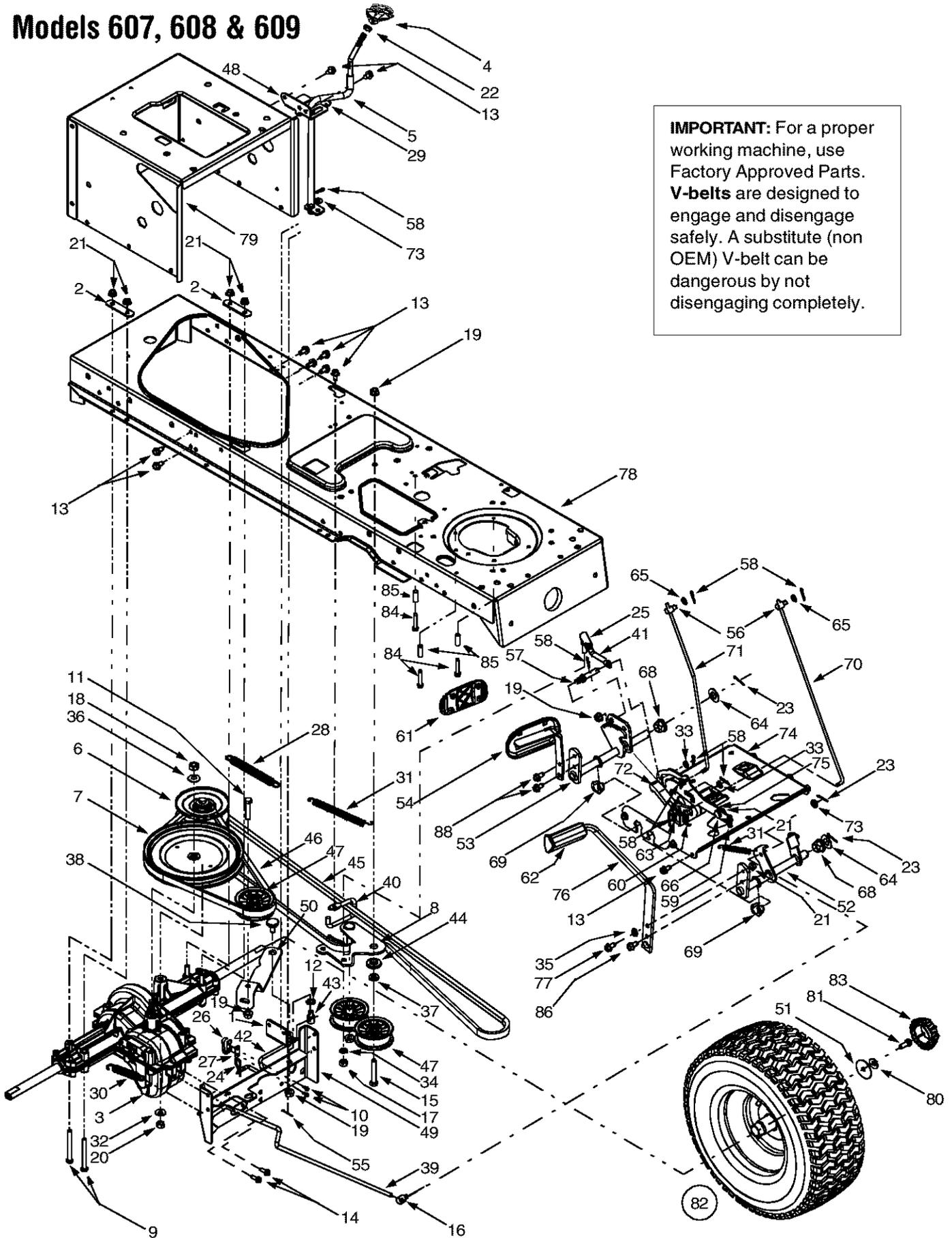
**IMPORTANT:** For a proper working machine, use Factory Approved Parts. **V-belts** are designed to engage and disengage safely. A substitute (non OEM) V-belt can be dangerous by not disengaging completely.
