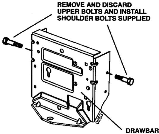
2. Align support assembly pin with hole in drawbar and hang assembly over the shoulder bolts.
