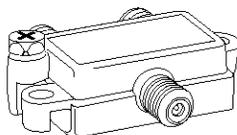
In order to watch one channel while you record another, you must connect the 2 Way Splitter correctly and change the TV to the channel you want to watch while the DVD Recorder stays on the channel you want to record. Operation with cable boxes varies. Not applicable with satellite receivers.
