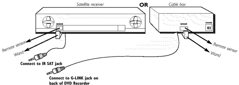
7. Place the wand in front of the remote sensor, approximately one inch away from the remote sensor.
