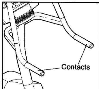
When your pulse is detected, the Heart Rate indicator above the right display will begin to flash, one or two dashes (--) will appear in the right display, and then your heart rate will be shown. For the most accurate heart rate reading, hold the contacts for at least 15 seconds.
