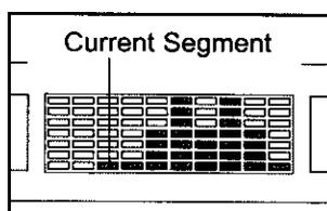
When only three seconds remain in the first segment of the program, both the Current Segment column and the column to the right will flash, a series of tones will sound, and all stepping speed settings will move one column to the left. The
