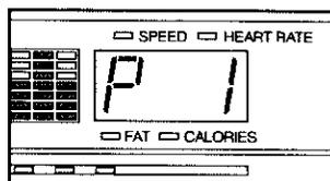
When a workout program is selected, the matrix will show the first seven stepping speed settings of the program. The left display will show how long the program will last.
