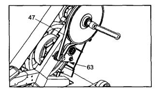
Next, turn the indicated M10 Nylon Locknut (63) until the Drive Belt (47) is properly tightened. Then, reattach the right side shield.
