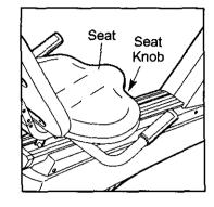
seat knob snaps into one of the holes in the seat rail.
