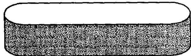
INSTALL BIDIRECTIONAL BELTS IN EITHER DIRECTION
