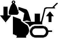
Weight Transfer Lift Handle To Engage
