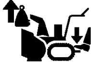
Weight Transfer Depress Pedal To Disengage
